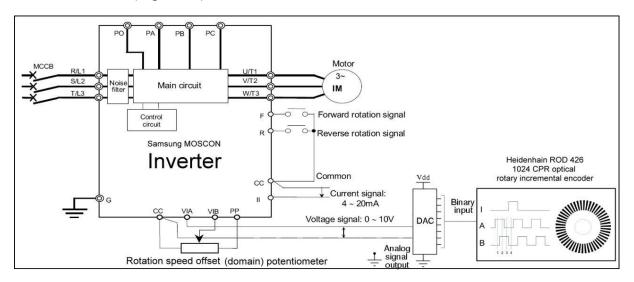
Figure 4. Schematics of the installation
