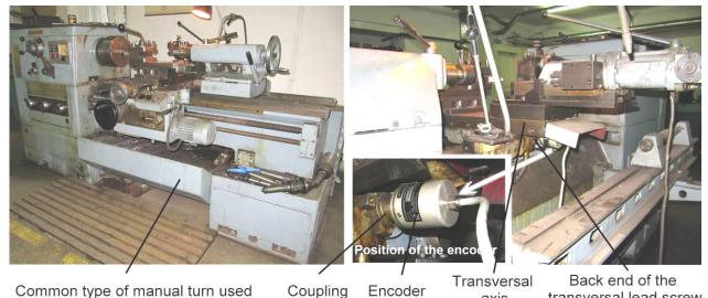
common type of manual turn used Coupling Encoder axis transversal lead screw
