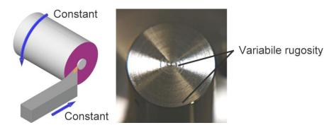
Figure 1. The fix rotation speed creates variable rugosity
