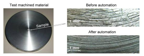
Figure 5. The resulted comparative surface after automation
